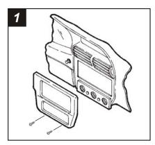
Disconnect the negative battery terminal to prevent an accidental short circuit. Using a small set of pliers, grasp the retaining clip on the back of the gear shifter handle and remove the clip. Remove the gear shifter handle. Unclip the center console and remove. Remove (2) 7mm hex-head screws exposed under the climate controls. Unclip the radio trim bezel and remove. Remove (2) 7mm hex-head screws securing the factory head unit and disconnect the wiring.
